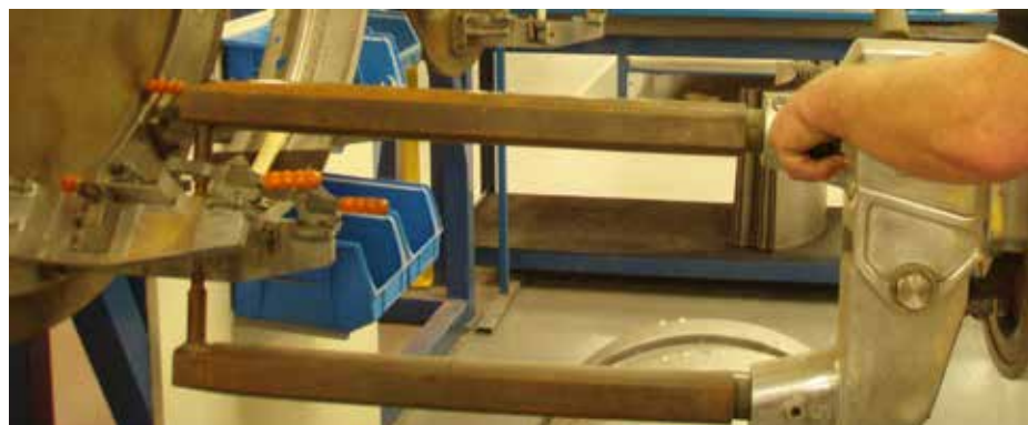
Figure 7.2 — Portable suspended spot welder
